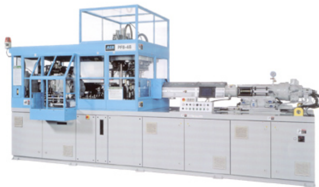
Figure 1: Actual Image of a Plastic Bottle-Molding Machine
